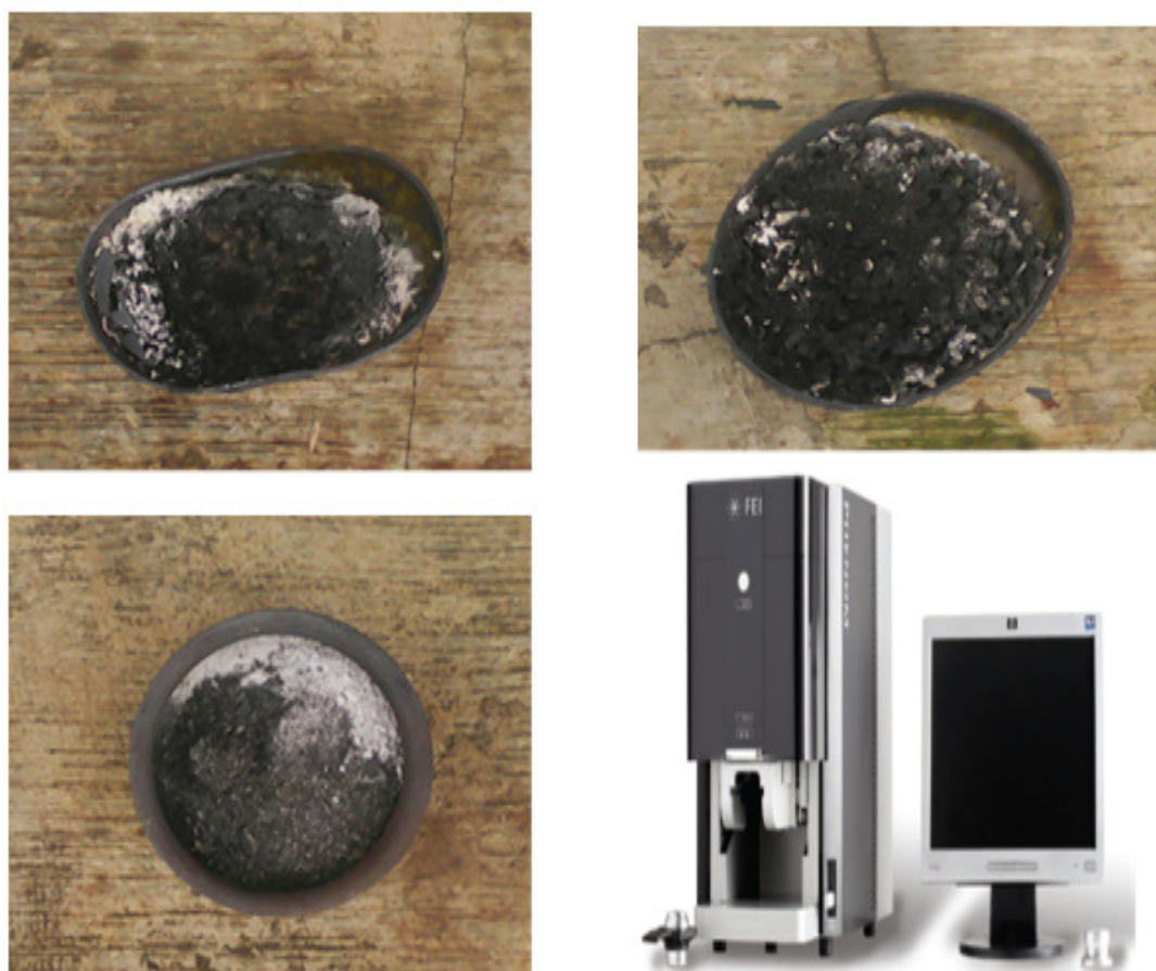
Figure 2: Characterization of Sawdust Char (a) Sawdust char produced from sawdust and KOH (b) Sawdust char produced from sawdust and NaOH (c) Sawdust char produced from sawdust and \text{Ca}(\text{OH})_2 (d) Microscope (SEM), Make: Phenom proX SEM, Model No: 800-07334)
