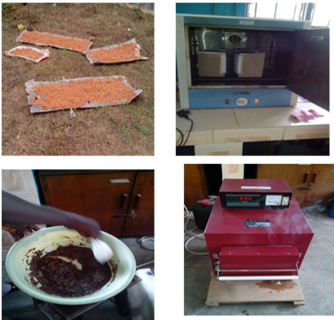
Figure 1: Preparation of Sawdust Char (a) Sun Drying of Sawdust (b) Drying of Sawdust in an oven (c) Preparation of Sawdust with KOH (d) Furnace in Operation at 500°C
