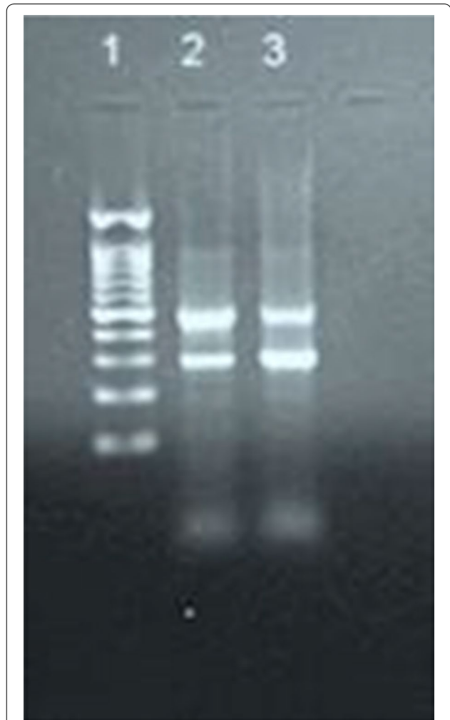
Fig. 1 Polymerase chain reaction amplification of Plasmodium vivax DNA of the blood sample from the patient showing amplification of 499 bp amplicon characteristic of P. vivax . Lane 1: Molecular weight standard 100 bp, lane 2 positive P. vivax control, lane 3: patient's sample
