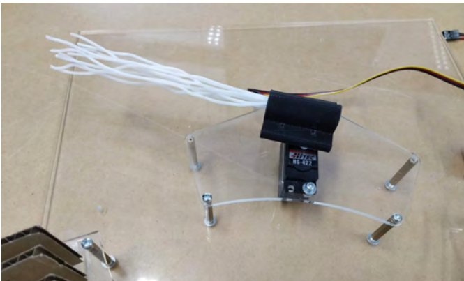
Fig. 6. Scraping apparatus made of 10 fine dowels, made of ABS filament.
