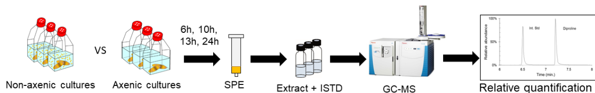
Figure 20: Target diproline analysis: general experimental setup. Medium of axenic and non-axenic MT-cultures under different conditions at different time points (see paragraphs 9.3.2-9.3.5) were extracted on SPE cartridges and the samples were measured with a single quadrupole GC-MS (Thermo Scientific® ISQ). Diproline was normalized to the internal standard caffeine.
