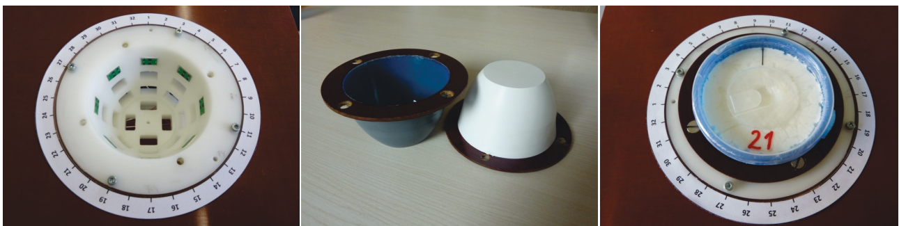
Figure 2. Antenna array (slide-in system) for 28 antennas equipped with the upper 8 antennas (left), two samples of cast contact layers (middle) and the finished measurement setup including a rotatable breast phantom
