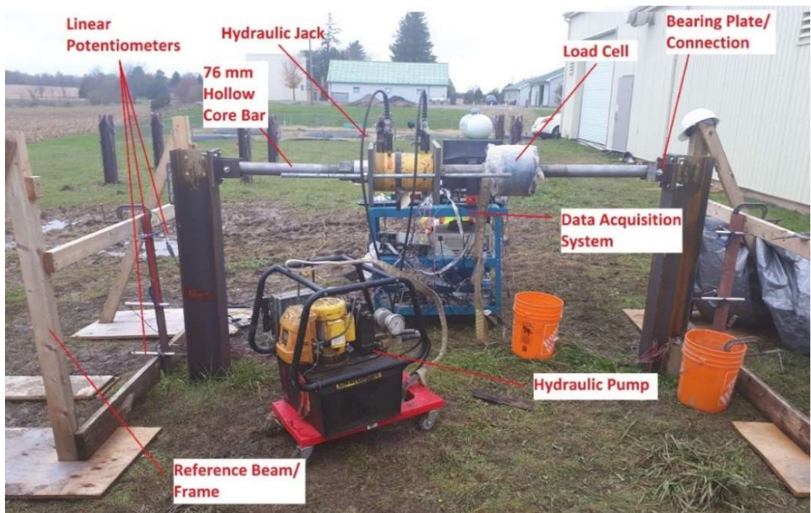
Figure 4-1: Lateral load test setup for two piles tested simultaneously.
