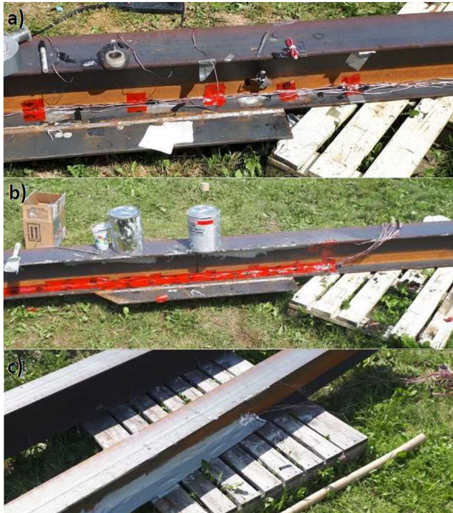
Figure 3-7: Application of a) sealant, b) construction grade sheathing tape and c) ceramic epoxy for strain gauge protection.
