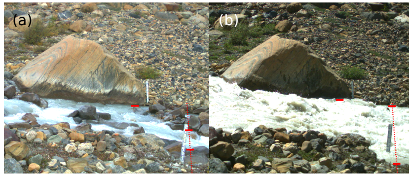
Figure 11. The width measurement at low (a) and high (b) discharges. The left line is the water level at the boulder station. The dashed line is the cross section and the right ticks are the detected flow edges.
