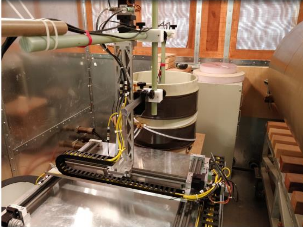
Figure 2.2-2: The experimental setup. In the foreground is the robotic system used to collect the field data over the volume of the dB/dt coil, the cylindrical system in the midground. The grey regions contain the wire windings of the coil.
