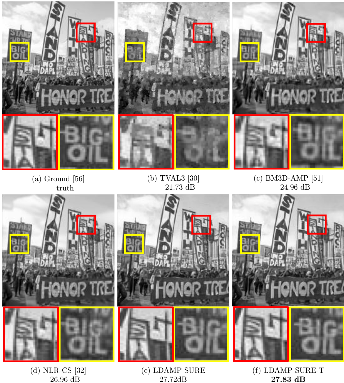
Figure 3.2: Reconstructions of 180 \times 180 test image with i.i.d. Gaussian matrix with M/N = 0.25 sampling rate.
