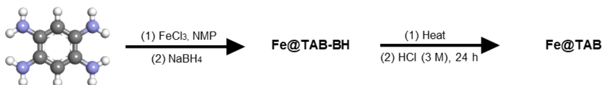
Figure 2.11. Schematic representation of the synthesis of Fe@TAB.
