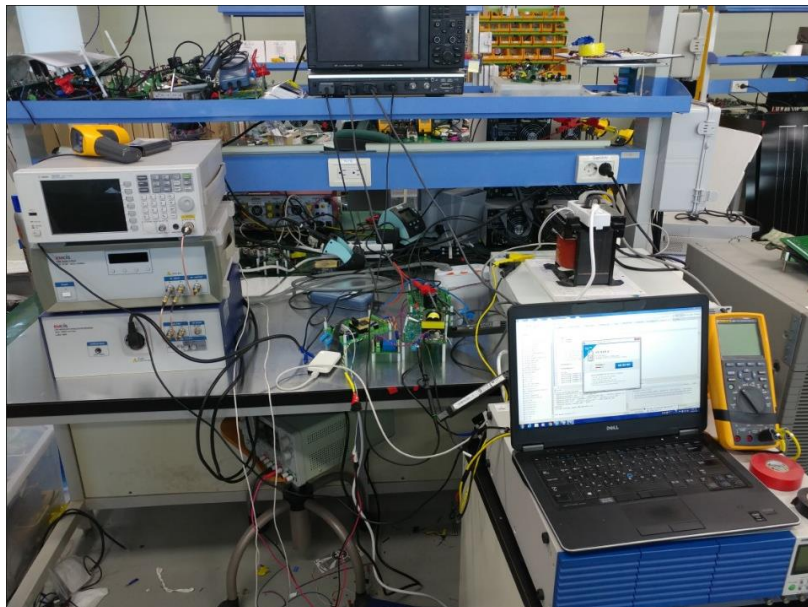
Fig. 59 Experimental setup of 100 W prototype power converter.
