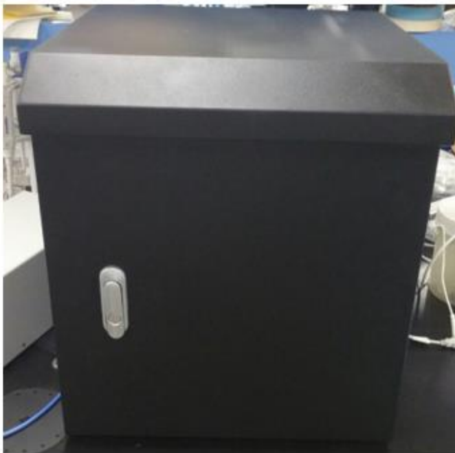
Figure 4.8. (A) Image of disc analyzer for absorbance and chemiluminescence detection. (B) Light blocking black box for containing disc analyzer.
