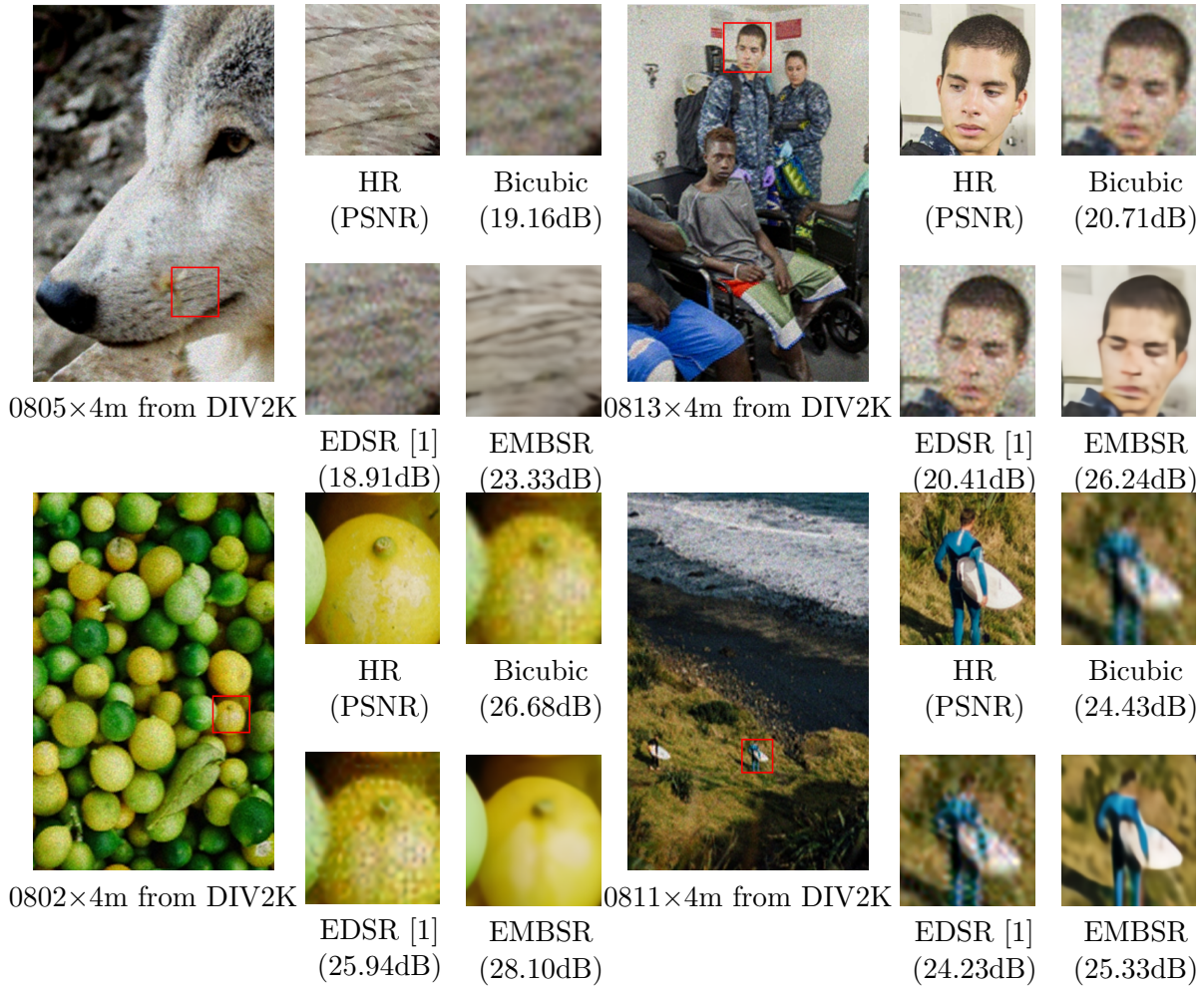
Figure 3.6: SR results of Track 2 in NTIRE 2018 challenge (unknown downsampling \times 4 with mild blur and noise). Our EMBSR yielded superior PSNR and image quality to EDSR and efficiently tackled SR problem with mild image degradation.
