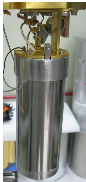
Figure B.2 Photograph of JPC mounted on the mixing chamber stage in dilution fridge.
