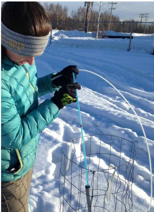
Figure 2.8. Checking permafrost tubes. The separated lines of blue in the right hand photo indicate areas of frozen ground.
