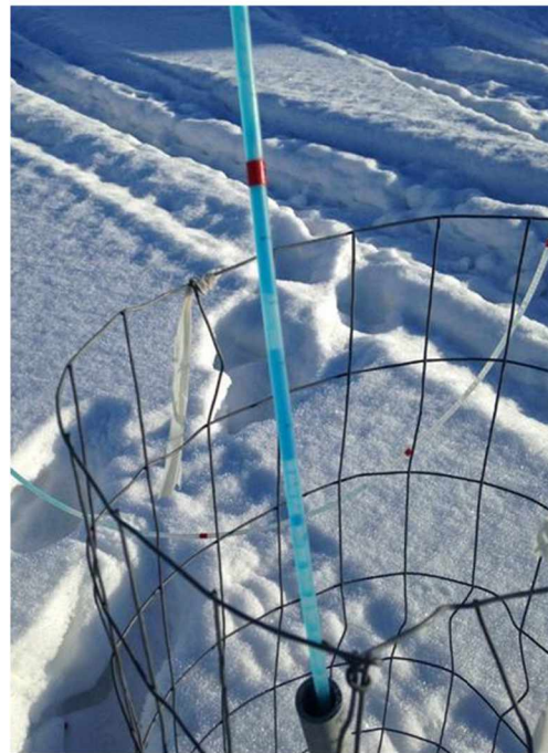
Figure 2.8. Checking permafrost tubes. The separated lines of blue in the right hand photo indicate areas of frozen ground.
