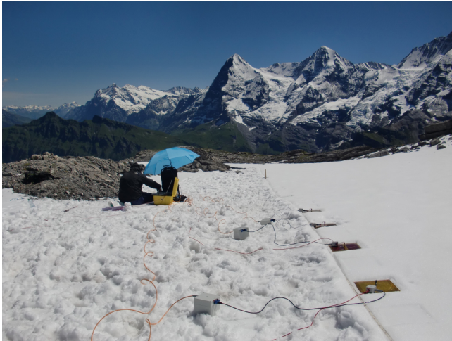
Figure 2. Photograph of the measurements at profile B-SCH (Schilthorn area) in July 2016 with the Chameleon measurement device. The four plate electrodes are lying in line on the snow surface. The larger yellow box is the base unit which is connected by cables to the electrodes with the cubic grey remote units in between.
