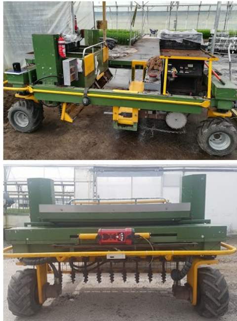
Figure 1.1.: Current System used by Lilies by Blewden . The first image provides an overall view of the system, while the second image shows the ten augers used for the process.
