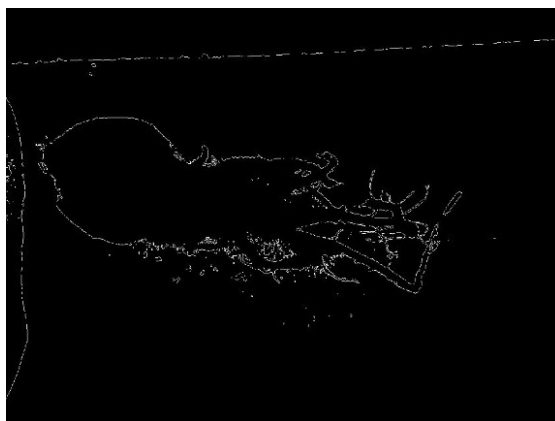
Figure 2.2.: Sample binary image with its edges isolated using a MATLAB sobel edge detection algorithm
