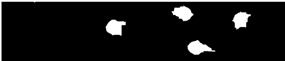
Figure 3.7.: Eroded binary image with only the bulb heads present, with some remnants of their respective stem structures.
