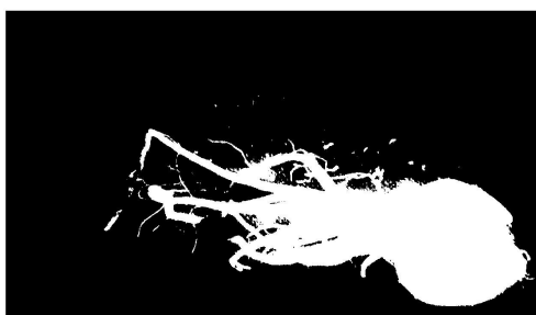
Figure 2.1.: The sample image of the lily bulb being isolated from its respective background using Otsu's method of global thresholding
