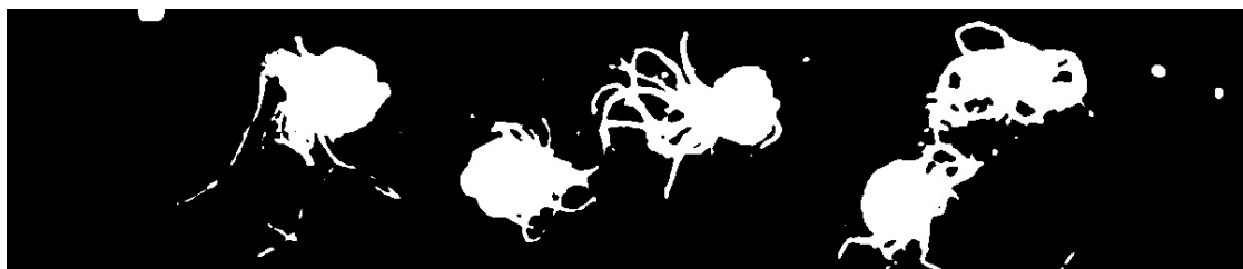
Figure 3.18.: Sample image depicting the issue with otsus threshold present in some of the test samples. The rightmost bulb has a cavity present that would propagate with further erosion, deteriorating its shape characteristics.
