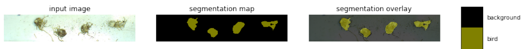
Figure 3.19.: Example output used with a pre-trained neural network on a sample bulb image. The outputs are seen as birds since the network had not been trained for bulbs.
