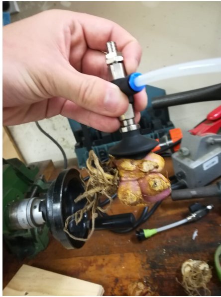
Figure 4.1.: Example of a bulb being lifted using a suction cup end effector. The head centroid is crucial for an optimal lifting procedure
