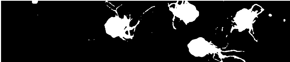
Figure 3.5.: Otsu's global threshold method used on the blue filtered sample image displayed in Figure 3.3
