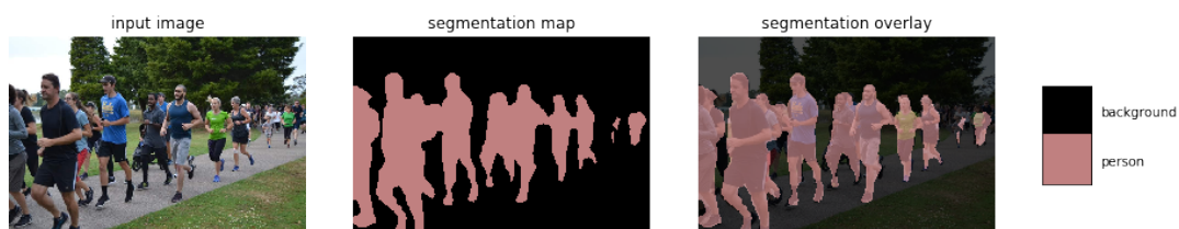
Figure 2.4.: Sample image processed using a Deeplab semantic segmentation using the MobilenetV2 as the main pre-trained network (Sandler et al., 2018). Runners are accurately segmented as people.
