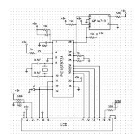
Fig. 4. Circuit built for the goniometer.
