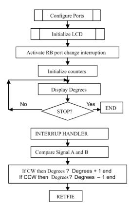
**Fig. 6.** Simplified flow diagram of the algorithm implemented. The detection of CW and CCW is based on the comparison between the interruptions Ii-1, Ii and the Ii+1. So the direction detection is based on the state of the PORTB in three different states of the input signal (three transitions).
