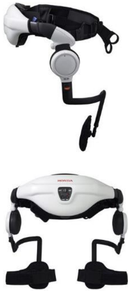
Figura 59. Honda Walking Assist
