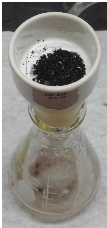
Figure 52 0CNC – 0G sample during filtration. Notice the brittle appearance of the polymer.
