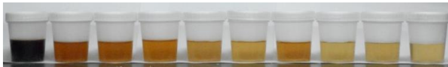
Figure 46 From left to right, 5CNC – 0G sample filtrate from each step, after 30 min of centrifugation
