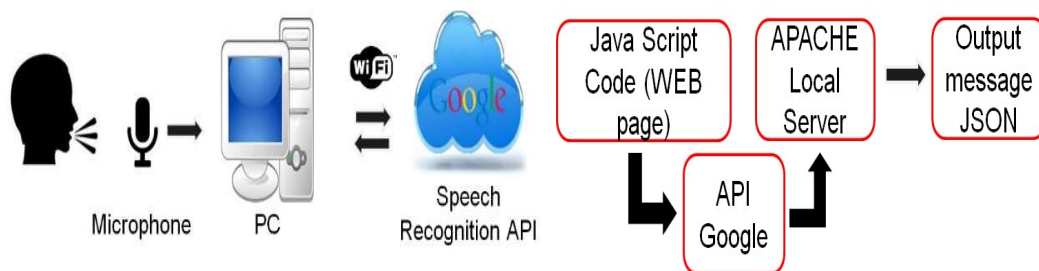
Fig. 4.3-3. Functional Voice Recognition Module and Components Speech Recognition Module.
