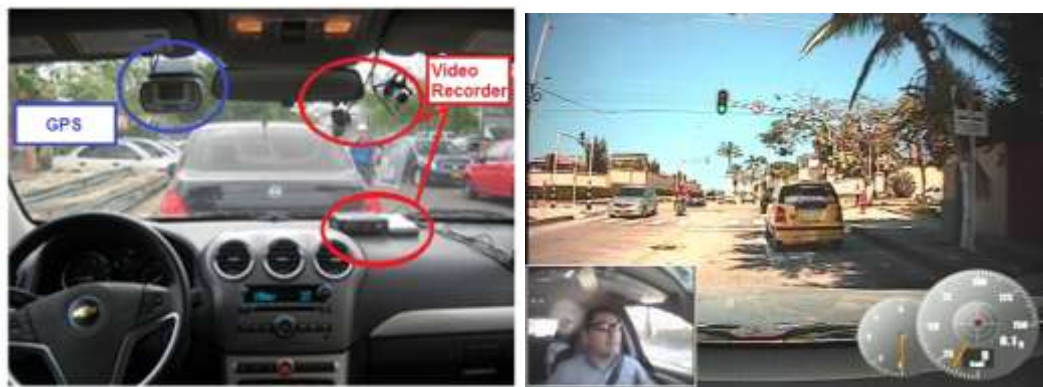
Fig. 5.2-4 - Adapted Prototype for Vehicle Telemetry Data Acquisition and Video Recording
