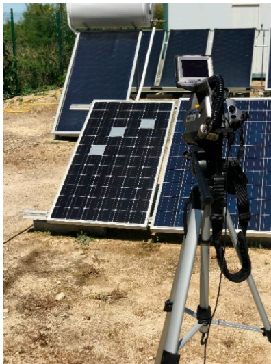
Figure 3. Position of the thermal camera in front of the covered PV cells E-3, C-4, and B-6.
