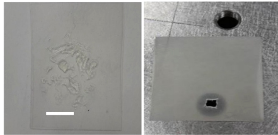
Fig. 3. Crude approaches to simulate the cataract effects with a model eye. Some random patterns drawn on a plastic thin film using glue (left) and a piece of paper with a 2 mm aperture (right). The scale bar on the left represents 5 mm.
