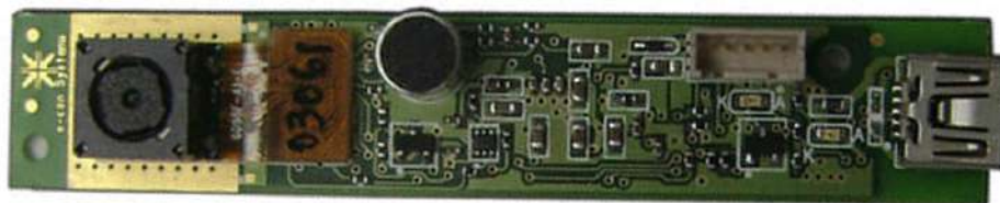
Figure 4.2: Embedded e-CAM51_USB - 5 MP OEM USB Camera Module [43].
