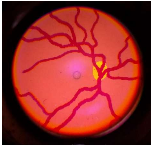
Figure 5.9: Eye phantom model image captured using Nexus 5X smartphone and the current EFS optical system prototype. Aliasing is very reduced when comparing to the plain millimeter paper images captured, despite revealing some chromatic aberrations closest to the borders of the eye model.
