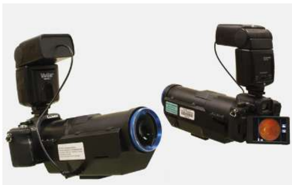
Figure 3.2: Hand-held, low cost fundus camera prototype developed in [26].
