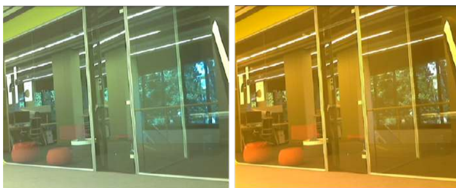
Figure 5.5: CameraApp has a white-balance controllable feature, that can be adjusted by the user before image capture, by adjusting the value of the white-balance Scrollbar implemented in the Settings Menu.
