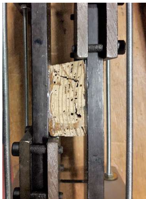
Figure 6: Rupture of the sample by shear parallel to grain test [4].
