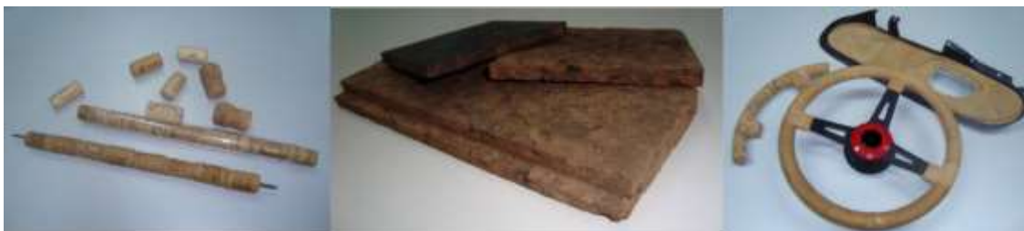
Figure 2: Typical applications of cork from isolation, fabric textiles, bulletin boards, automobile components and stoppers to heat-shields of spacecrafts [24].
