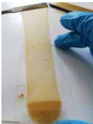
Figure 8: Cork-based electrolytic membrane showing its elastic capabilities.
