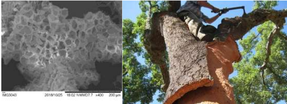
Figure 1: Obtained SEM image of untreated cork powder, and the harvesting of cork [22].
