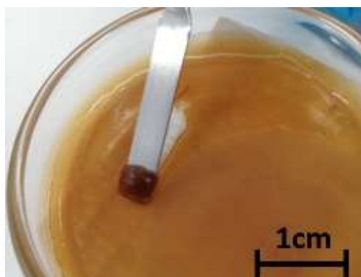
Figure 7: Sample of cork-resin resulting from the dissolution and neutralization steps without adding a binding agent.
