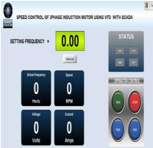
Figure 2-5 - User interface provided for the IoT of an induction motor [24].
