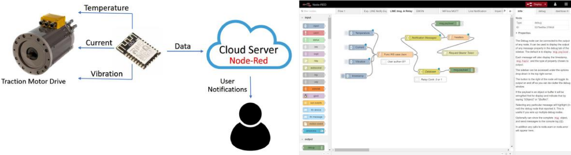
Figure 2-7 Wireless Internet of Thing traction motor drive block diagram (left) and Node-Red cloud platform (right) [26].
