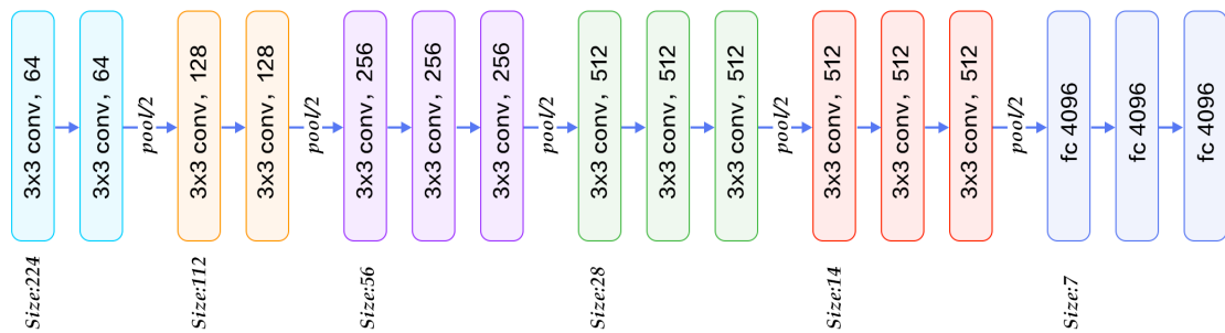
Figure 2.13: The Architecture of the VGG network. The Softmax layer with 1000 nodes at the output is omitted at the end, for simplicity.
