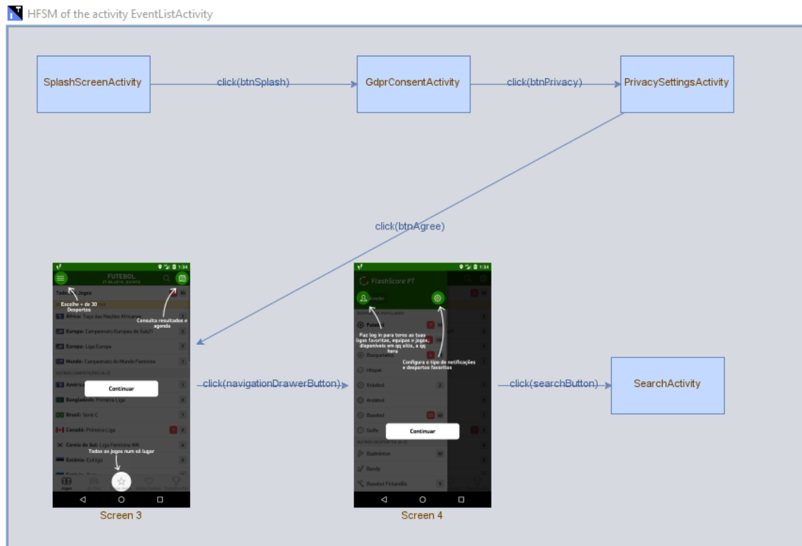
Figure 5.3: The second level of the HFSM detailed for Activity EventListActivity.
