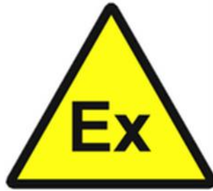
Figure 3.5 – Warning sign for places where explosive atmospheres may occur. Adapted from Directive 1999/92/EC.
