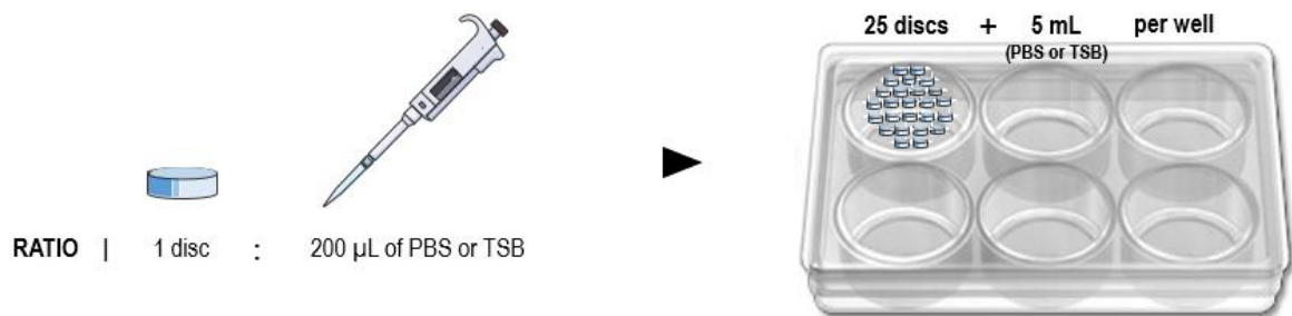
Figure 7 – Schematic representation of the discs extracts preparation.
