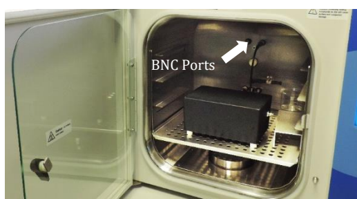
Figure 5.2. Incubator with the sensor case evidencing the BNC Ports installed on the incubator wall
