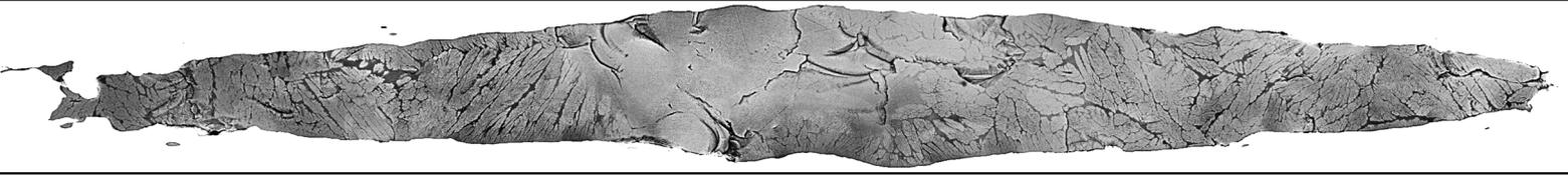
Figure 86 – Stitched BSI images for inclusion B of the sample from slab 6. Depth and length of the inclusion are  $2194\mu\text{m}$  (18% of the final slab thickness) and  $866\mu\text{m}$  respectively. Rolling direction from left to right.
