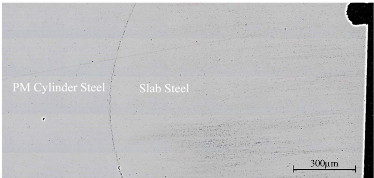
Figure 33 – Detail of the sample from slab 2 created with 50x optical microscopy images. Boundary between the steel slab and the powder metallurgy cylinder highlighted.
