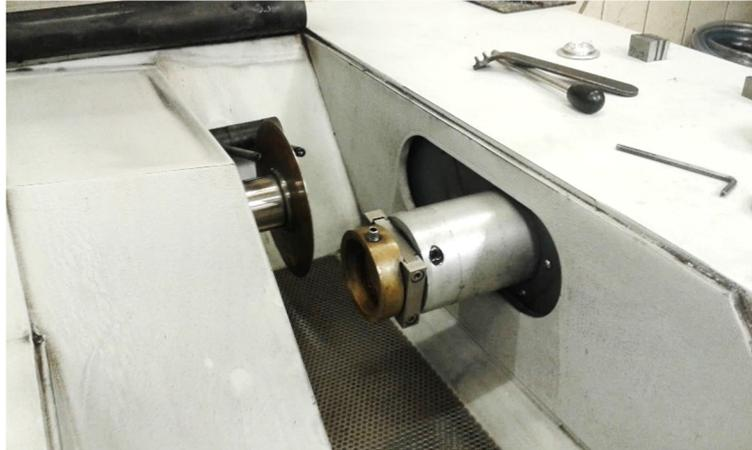
Figure 27 – Struers Accutom-5 used in the sample cutting process.
