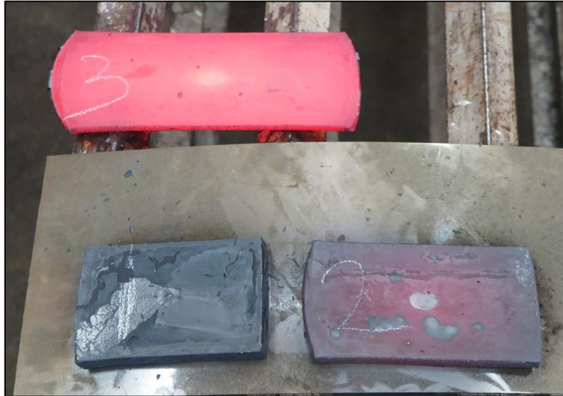
Figure 26 – Slabs 1 (lower left corner), 2 (lower right corner) and 3 (top) after hot rolling. PM cylinders visible in the centre of the slabs.
