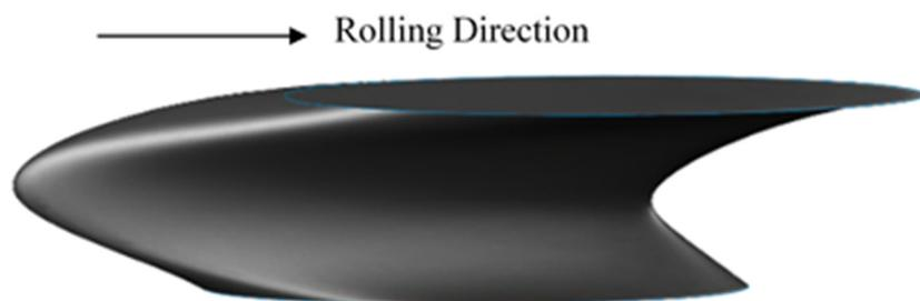
Figure 28 – Representation of the expected deformation of the rolled cylinders (not to scale) [9].
