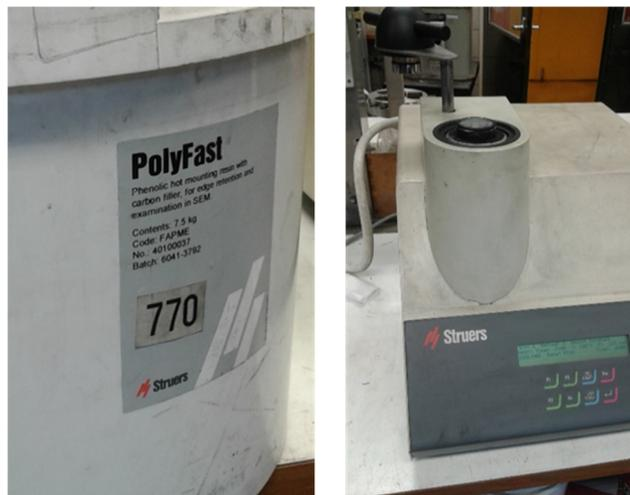
Figure 29 - Struers PolyFast carbon-filled phenolic resin (left) and Struers Protonpress 10 (right) used in the sample mounting.
