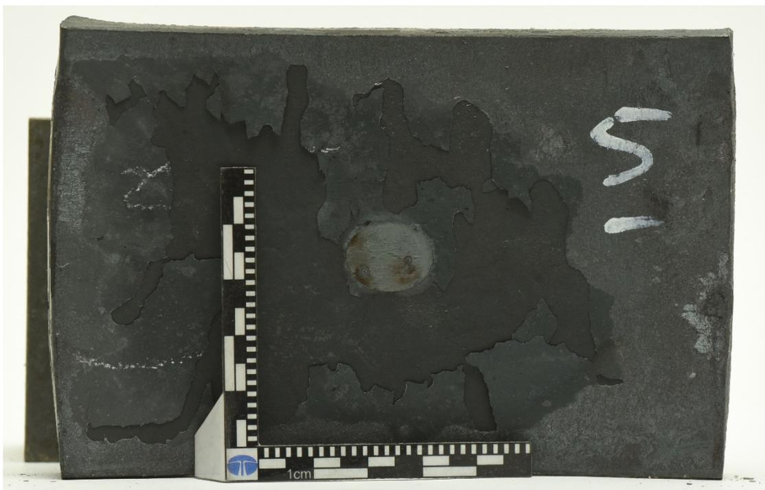
Figure A2 – Steel slab after the 20% thickness reduction lab scale hot rolling scheme. PM cylinder visible in the centre of the slab. Example taken from slab 5.
