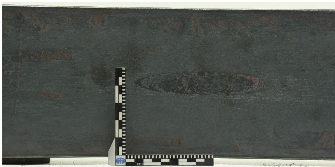
Figure A5 – Steel slab after the 85% thickness reduction lab scale hot rolling scheme. PM cylinder visible in the centre of the slab. Example taken from slab 12.
