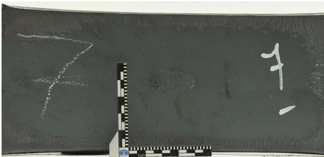
Figure A4 – Steel slab after the 60% thickness reduction lab scale hot rolling scheme. PM cylinder visible in the centre of the slab. Example taken from slab 7.
