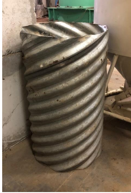
Figure 3.12 Corrugated steel pipe used as a casing in this testing program
