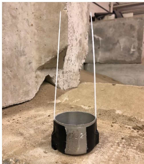
Figure 3.25 Typical density tin used to determine final density of the poorly graded clean sand
