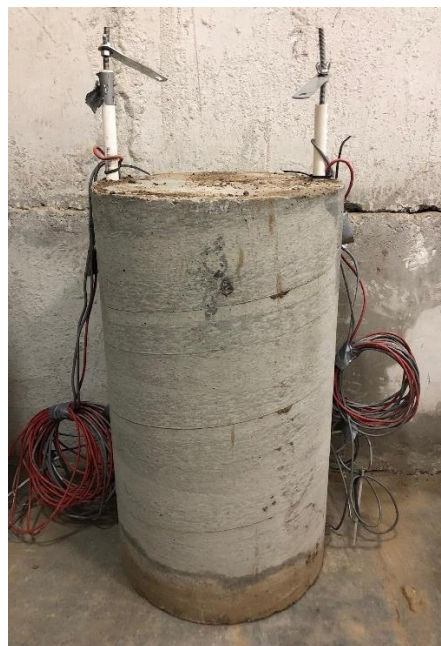
Figure 3.10 Final model drilled shaft foundation used during testing
