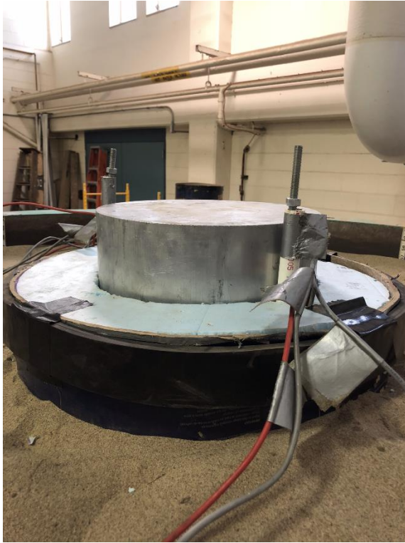
Figure 3.11 Reinforcement used to support the free end of the commercial sonotube casing
