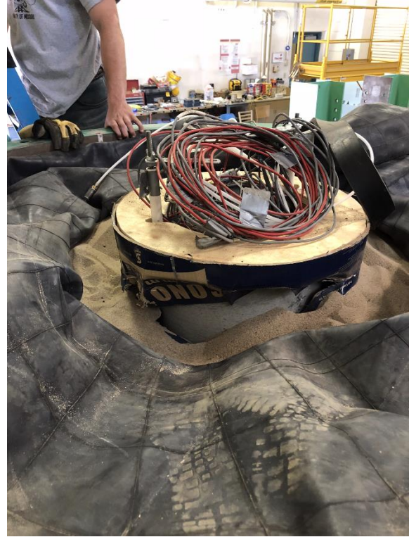
Figure 3.11 Reinforcement used to support the free end of the commercial sonotube casing
