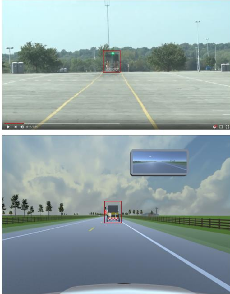
Figure 10: Calibrating the sight distance in Unity. Top: the AFAD device at a known distance of 250 ft. Bottom: The Virtual AFAD at the same distance.
