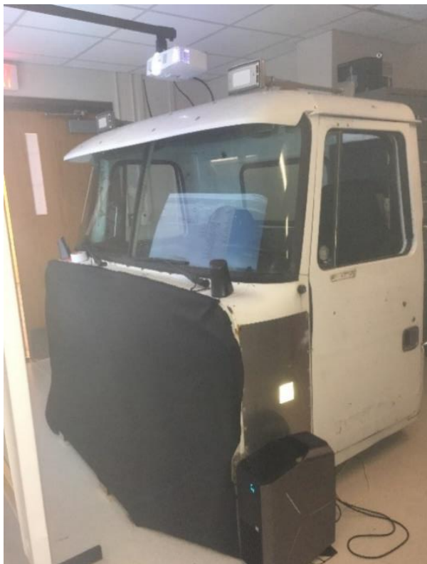
Figure 4: The Zou Sim Truck Simulator (Clockwise from top right): View of simulator during testing. The ZouSim truck simulator with the Unity Editor projected on screen. The Logitech G920 steering and pedal inputs. View of simulator "under the hood."
