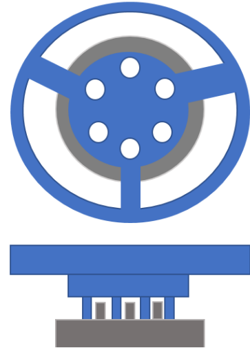
Figure 5: Salvaged steering wheel (in blue) and adapter attached to the Logitech G920 (in grey).
