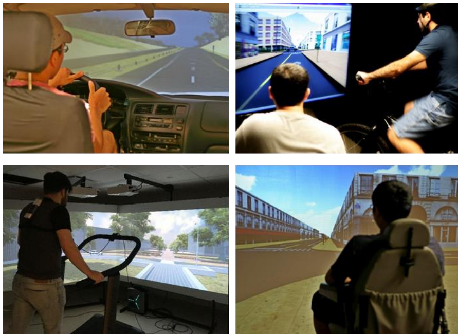
Figure 2: The ZouSim Simulator Suite. Clockwise from top left: Car Simulator, Bike Simulator, Wheel Chair Simulator and Pedestrian Simulator
