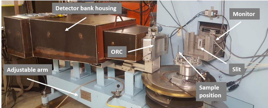
Figure 3.5. Photo of the two-axis powder neutron diffractometer located at D-port at MURR with several major components labeled (e.g., oscillating radial collimator ORC). Courtesy of Z. N. Buck [137].
