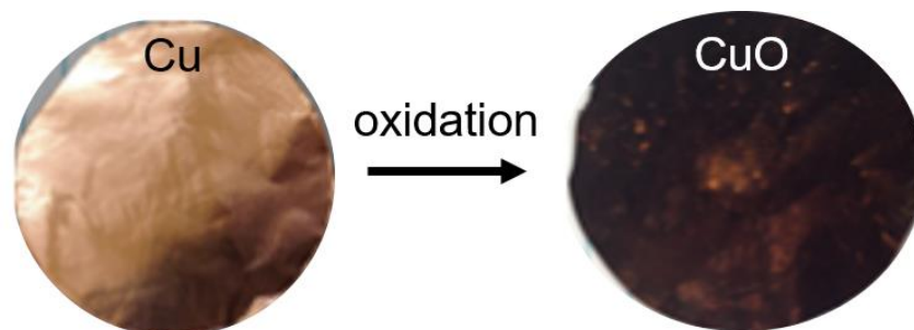
Figure 2.1. Photos of a 5-cm diameter, 12- \mu\text{m} thick copper foil (left) before and (right) after oxidation using the recipe developed by Liu et al. [98].
