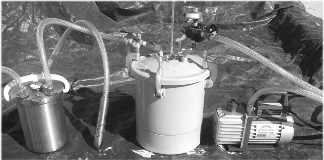
Figure 4.1. Images of the collection containers and probe used for the extraction of rumen fluid to be used in the continuous culture.
