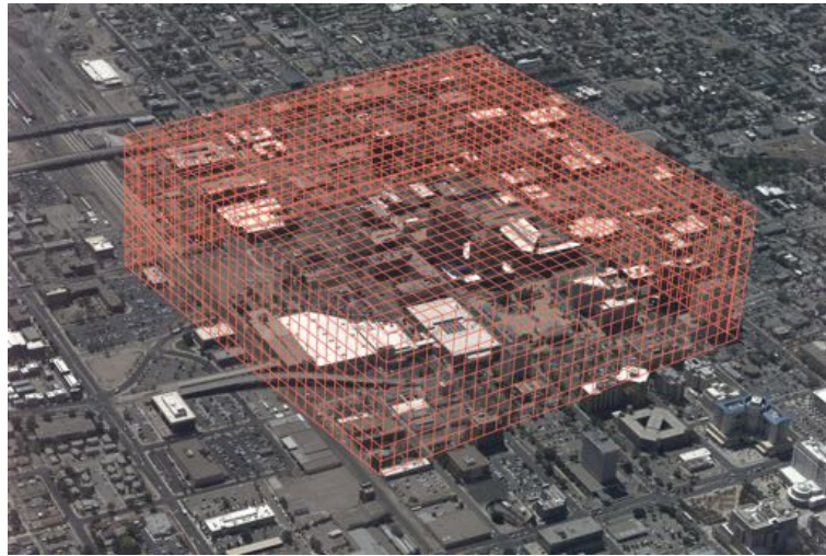
Figure 2.9: An example of Voxel Grid on the Albuquerque Dataset. Because of memory limitation is is often impossible to cover the whole scene at high resolution.
