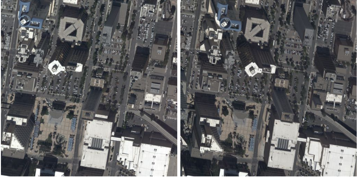
Figure 1.4: Example of motion parallax, side by side comparison of two different orthorectified views from Albuquerque Dataset, showing an obvious change of orientation of the tall buildings projections. .
