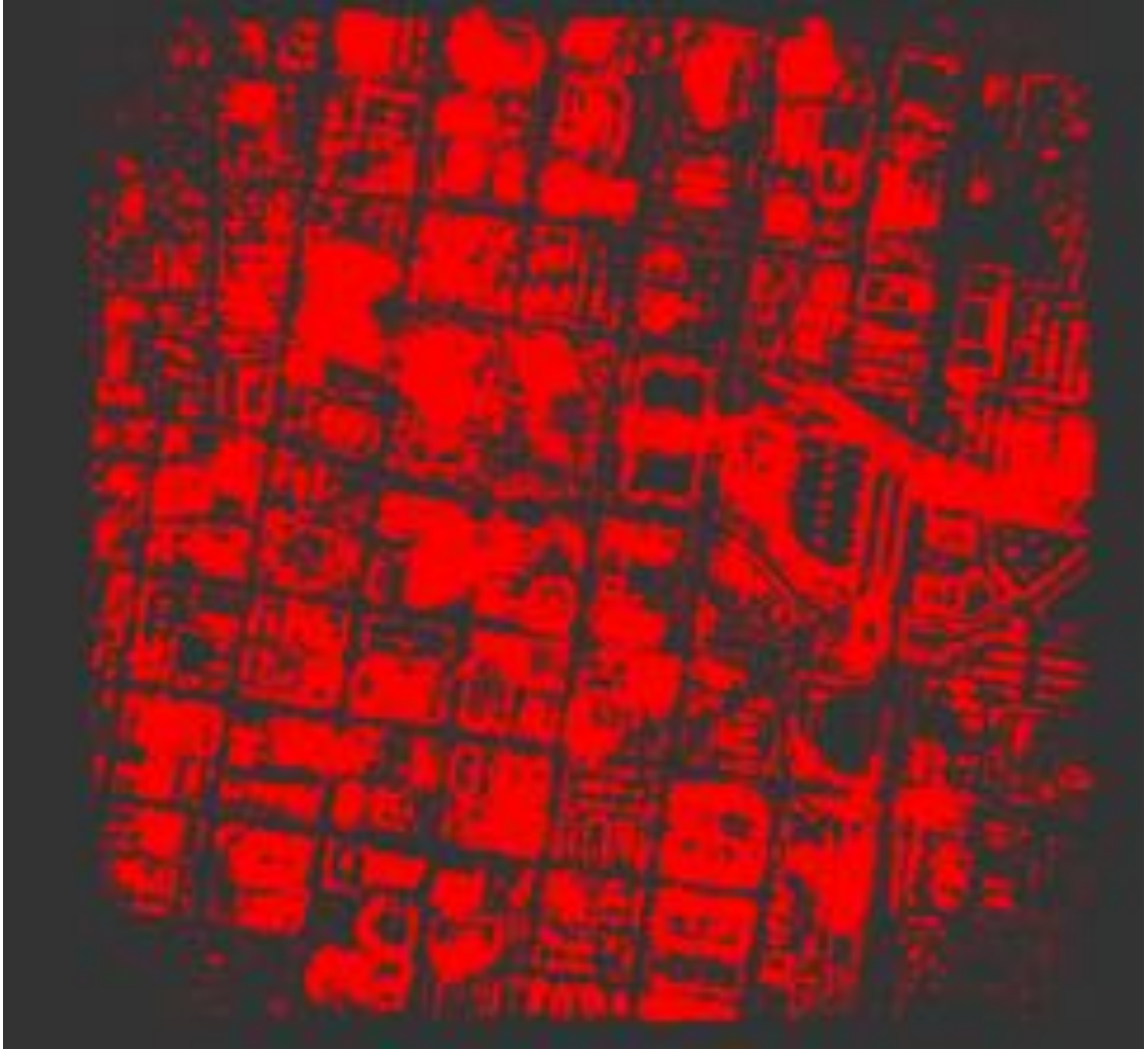
Figure 4.19: Screenshot of a point cloud of Albuquerque Dataset obtained with the vote accumulation thresholding method.
