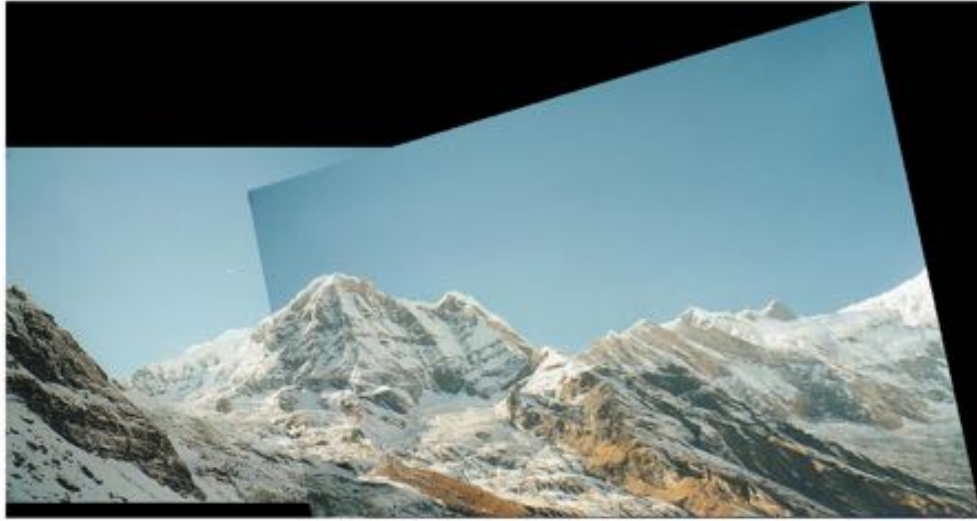
Figure 2.6: After applying the homography estimated with Direct Linear Transform and RANSAC. The target image is warped and overlaid on the reference image that remains unchanged. [27]
