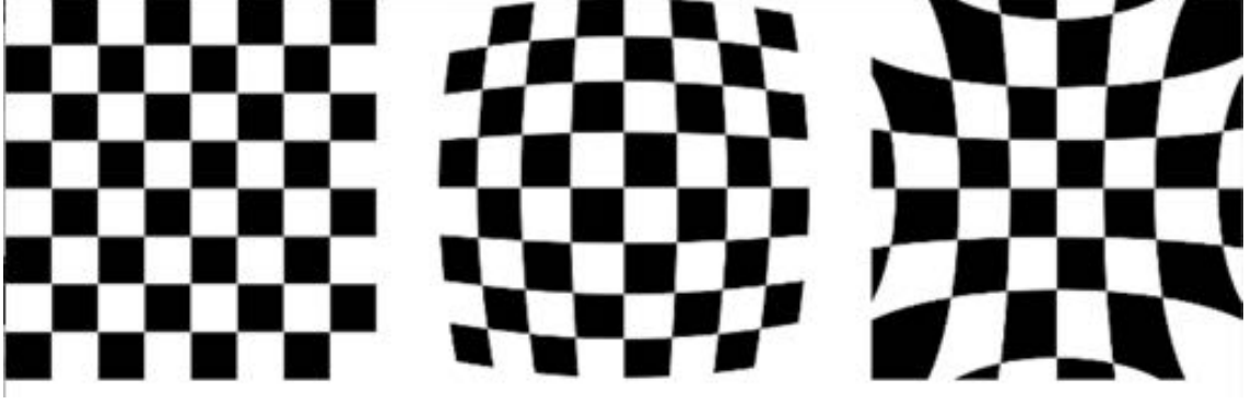
Figure 2.3: Left: No Distortion. Center: Positive Radial Distortion (Barrel) Right: Negative Radial Distortion (Pincushion)
