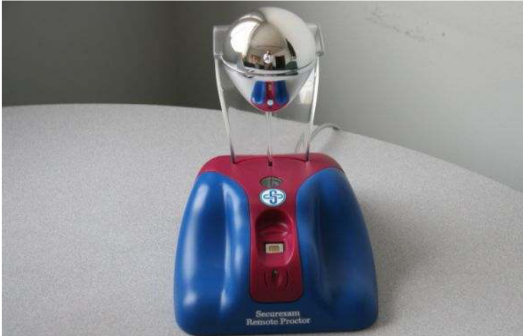
Figure 9: Software Secure Securexam Remote Proctor features finger print biometric device, microphone, and 360 degree camera (Software Secure Product Demos. Securexam Remote Proctor (2011)).
