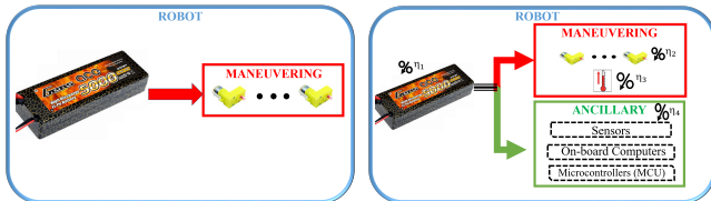
(a) Idealistic Battery Dissemination Model (b) Realistic Battery Dissemination Model
