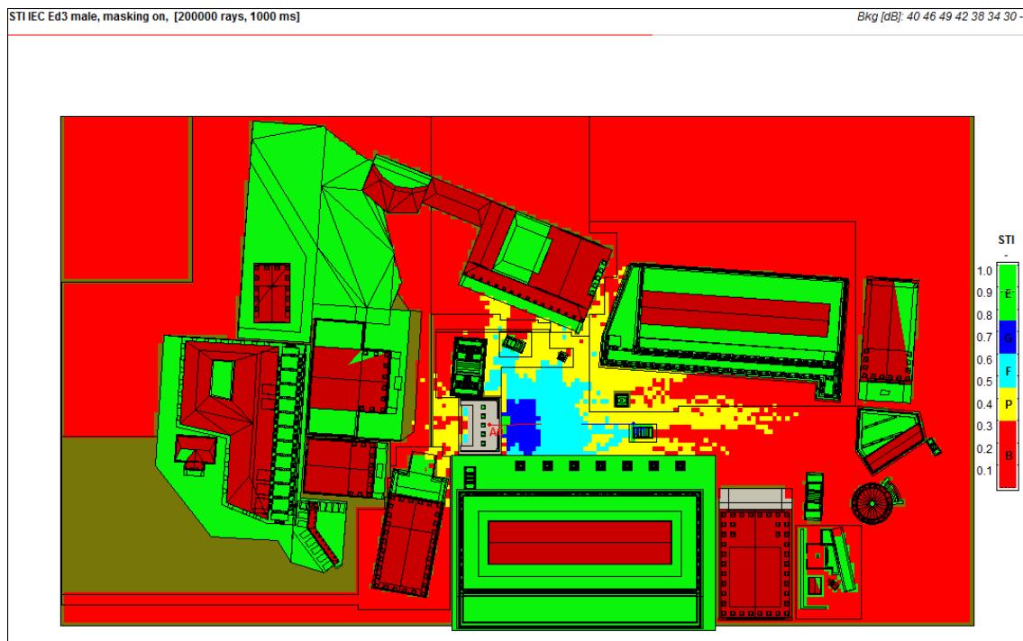
Figure 2. Results of STI analysis for speaker speaking from the Imperial Rostra with “typical audience” background noise. Green marks the area with the STI measure of 0.75–1.00 (‘Excellent’), dark blue marks the area with the STI measure of 0.60–0.75 (‘Good’), light blue marks the area with the STI measure of 0.45–0.60 (‘Fair’), yellow marks the area with STI measure of 0.30–0.45 (‘Poor’).
