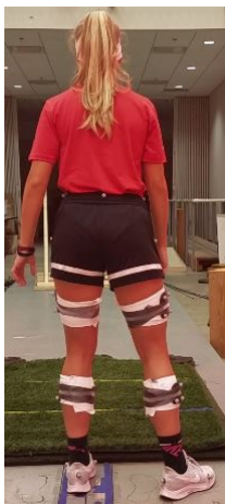
Figure 5. Retroreflective marker placement on the subject.
