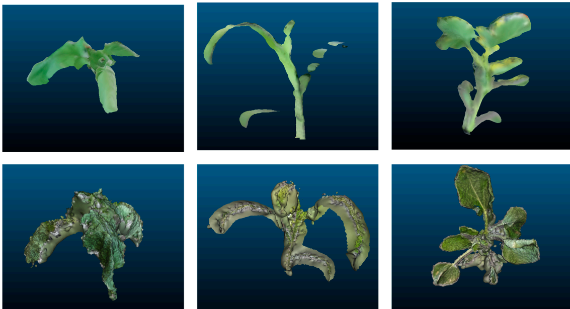
Figure 2. Examples from different perspectives of different crop models reconstructed using Kinect v2 ( top ) and photogrammetry ( bottom ) reconstruction methods.
