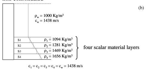
Figure 12a, b. Heterogeneous sediment stratum. (a): partially consolidated sediment; (b): non-consolidated sediment. See mechanical properties for poroelastic material layers in Table 3.
