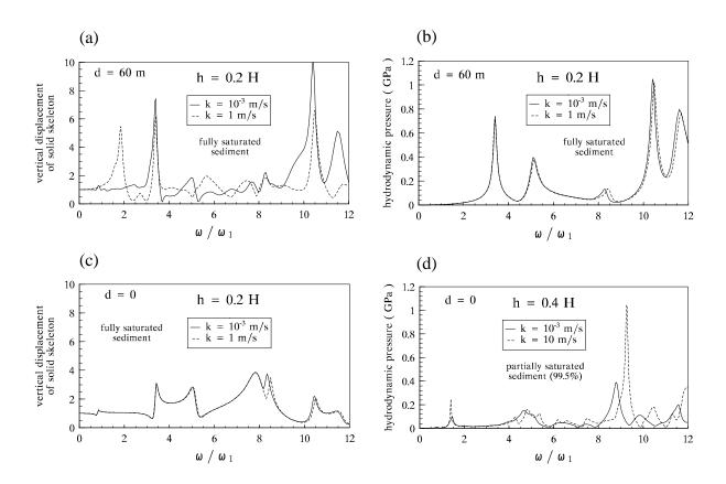
Figure 8a,b,c,d. Influence of sediment permeability. Local response of sediment to vertical excitation: vertical displacement of solid skeleton and hydrodynamic pressure for different points at water-sediment interface. d = distance from the wall face.
