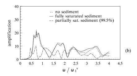
Figure 15a, b. 3-D Dynamic response of arch dams. Influence of sediments saturation degree. Upstream response at dam crest to ground motion: (a) upstream excitation (S wave); (b) vertical excitation (P wave).
