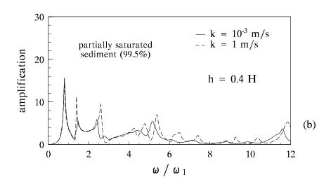
Figure 7a, b. Influence of sediment permeability. Horizontal amplification at the wall top to horizontal excitation for sediment thickness h/H=0.4.
