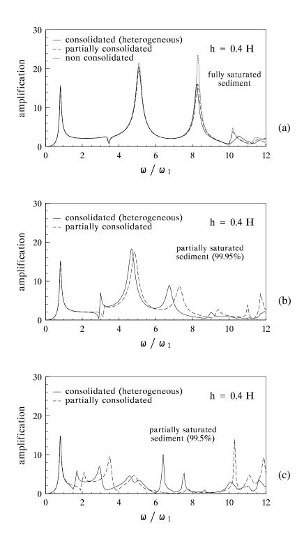
Figure 13a, b, c. Influence of consolidation degree. Fully and partially saturated sediments. Horizontal amplification at the wall top to horizontal excitation for sediment thickness h/H=0.4.
