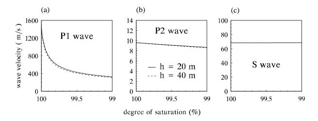
Figure 3. Wave propagation velocity amplitudes in the sediment vs. degree of saturation.
