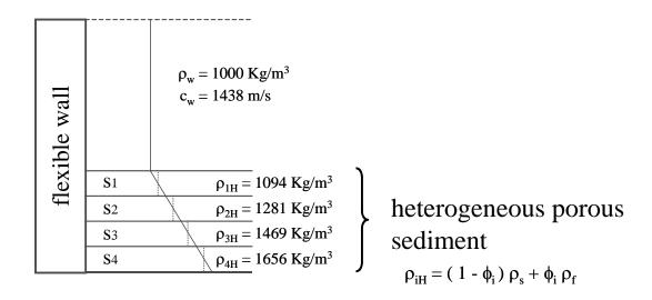
Figure 10. Heterogeneous porous sediment stratum. See Table 2 for mechanical properties for three different saturation degrees.
