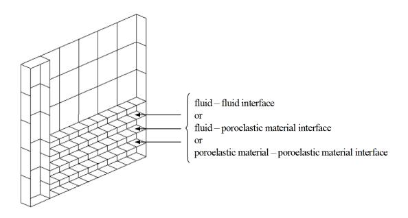
Figure 9. Heterogeneous sediment. Boundary Element discretization. See Table 1 for interface conditions.
