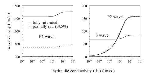
Figure 6. Wave propagation velocity amplitudes in the sediment vs. permeability.
