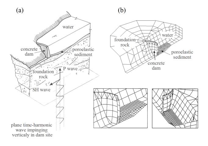
Figure 14a, b. 3-D coupled problem. Seismic response of arch dams. BE model for the coupled system.
