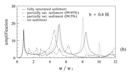
Figure 4a, b. Influence of sediment saturation degree. Horizontal amplification at the wall top to horizontal excitation for sediment thickness h/H = 0.2 and 0.4.
