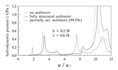
Figure 5. Influence of sediment saturation degree. Hydrodynamic pressure at z=0.6 H on the wall face. Vertical excitation.
