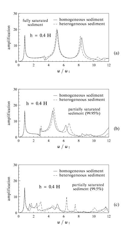
Figure 11a, b, c. Influence of sediment heterogeneity. Horizontal amplification at the wall top to horizontal excitation for sediment thickness h/H = 0.4.
