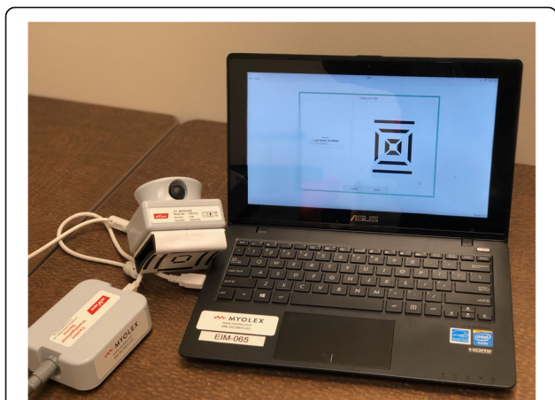
Fig. 2 Electrical Impedance Myography Legend: The EIM device consists of a laptop computer connected to a portable handheld sensor
