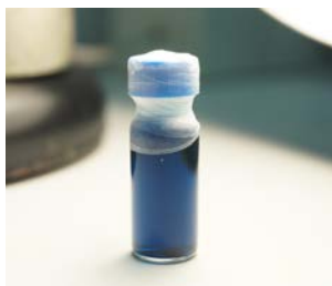
Figure 2.1: Acetates based solution with methanol:propionic acid 1:1 ratio
