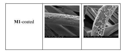
**Figure 2.** SEM images of uncoated and coated cotton and polyester weave. Coatings were prepared from 1% solutions of the respective polymers in *n*-hexane. The presence of a thin coating layer is evinced by edges and other layer irregularities, absent in images of the uncoated fibers.
