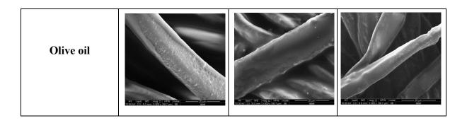
**Figure 5.** From left to right, SEM images of polyester, cotton and filter paper fibers after absorption of *n*-tetradecane (top) and olive oil (bottom). After draining of excess oil, no obvious smearing is observed for *n*-tetradecane; as opposed to olive oil.
