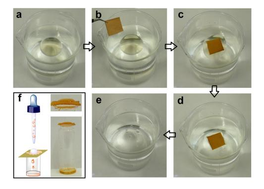
**Figure 7:** Selective oil removal: (a) *n*-tetradecane/water mixture; (b)-(e) oil is removed by soaking a **M1**-coated cotton sample. (f) Schematic representation of an oil/water phase separation by filtration over a hydrophobically coated substrate fiber (right); picture after filtration using a **M1**-coated cotton sample; water-phase retained on top (left). A small amount of dye was added to the oil phase to help with the visualization of the oil/water interface.
