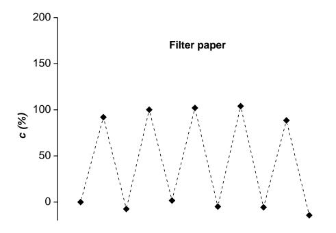
**Figure 6.** Recyclability of **M1**-coated fibrous substrates (cotton, polyester, filter paper) assessed by net oil absorption capacity, *c*. 5 *n*-tetradecane absorption/cleaning cycles were carried out (immersion, 10'; draining, 30'; rinsing in ethanol, 30'). Clean substrates were dried under vacuum at 30°C for 1h before re-weighting.
