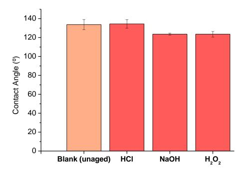
**Figure 4.** Chemical resistance of **M1** coatings on cotton against acidic (HCl 1M), basic (NaOH 1M) and oxidizing (H<sub>2</sub>O<sub>2</sub> 3% w/v) aqueous media: a) hydrophobicity of samples coated with **M1** and subsequently treated in the aging media; b) hydrophobicity of samples coated with previously aged polymer **M1**.
