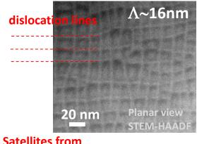
Highly ordered array of misfit dislocations produces a nanophase composite with distinct functional properties than bulk
