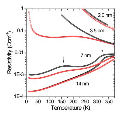
**Figure 8.** Resistivity versus temperature measured in thin LSMO/LAO films with different thickness at 0T (black) and 9T (red) applied magnetic field. The arrows indicate for the 7 nm thick film the maximum of magnetoresistance corresponding to the coexistence of low and high  $T_{\rm c}$  phases.
