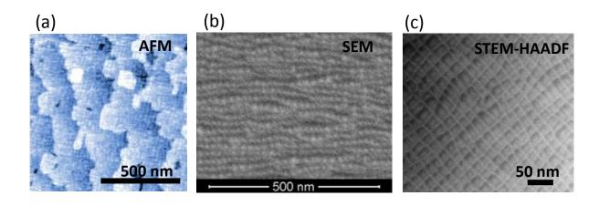
**Figure 1**. Planar view images of a 7 nm thick LSMO/LAO thin film with a well-developed misfit dislocation pattern as observed by AFM topography (a), orientation contrast SEM (b) and STEM taken at HAADF mode (c). In all cases the image contrast defines parallel lines that correspond to the position of the misfit dislocation cores parallel to [100] and [010] directions.
