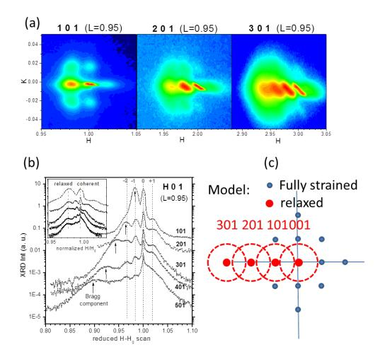
**Figure 5**. (a) HK Reciprocal space maps of H 0 1 (H=1, 2, and 3) reflections of the LSMO film with 7 nm thickness; and (b) linear H scans of the different reflections H 0 1, from H=1 to 5, the scans are shifted to coincide in the H position of the LAO substrate at H=1 (the inset shows the same scans reduced dividing by  $H_0$ ; along with (c) the corresponding model showing the overlap in the reciprocal space of fully strained and partially relaxed LSMO structures.
