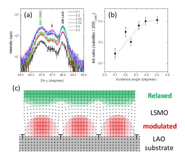
**Figure 7**. (a) In-plane diffraction  $2\theta$ - $\chi$  scans of the 200 reflection of the 7nm thick LSMO/LAO film using different incidence  $\omega$  angles from 0.1 to 0.5°. (b) Integrated intensity ratio of the satellite component versus the 200 LSMO Bragg reflection. (c) Model of the depth distribution of the outer relaxed LSMO and buried strained-modulated LSMO structure.
