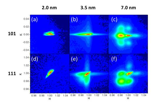
**Figure 6**. HK reciprocal space maps of the 101 and 111 reflections for the LSMO films with thickness 2.1 nm (a,d), 3.5 nm (b,e) and 7.0 nm (c,f). Maps were positioned at L=0.95 corresponding to the maximum of the LSMO contribution. (HKL in LAO reciprocal lattice units)
