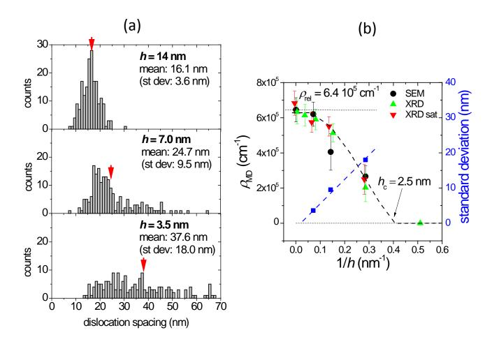
**Figure 4**. (a) Distribution histograms of the separation between consecutive misfit dislocations measured from the SEM images of the films of different thicknesses; and (b) dependence of the linear dislocation density versus the reciprocal film thickness (as measured by SEM (black symbols) and XRD: as estimated from the LSMO cell parameter value (green symbols) and from the satellite peak position (red symbols), along with the standard deviation of the distribution by SEM (blue symbols).
