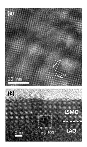
**Figure 2**. High-Resolution TEM images of a planar view (a) and cross-section (b) of a 7nm thick LSMO/LAO film. The cross-section shows a Burgers circuit around a misfit dislocation core at the film-substrate interface with a Burgers vector  $\mathbf{b} = a_{\text{LAO}}[100]$ .
