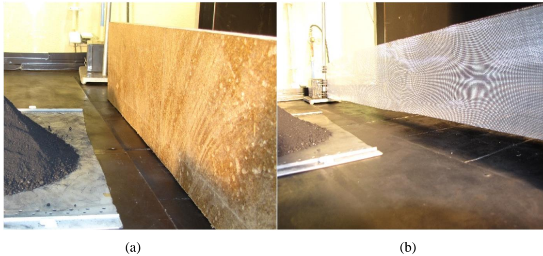
Figure 5. (a) Solid and (b) Porous barriers used in the wind tunnel experiments ( Z=2\text{ m} ).
